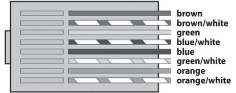
figure 4 - Type B RJ45 termination colour code
