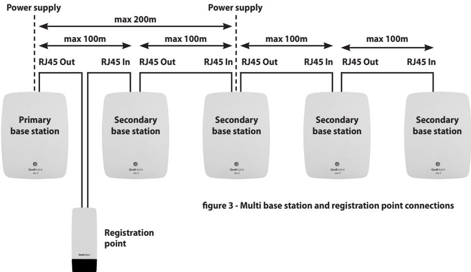
figure 3 - Multi base station and registration point connections
